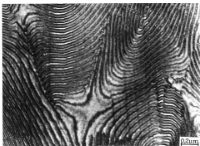
Figure 2. Higher magnification of lamellar morphology. The dark lines between the PS (dark) and PnBMA (light) domains correspond to the interface.
