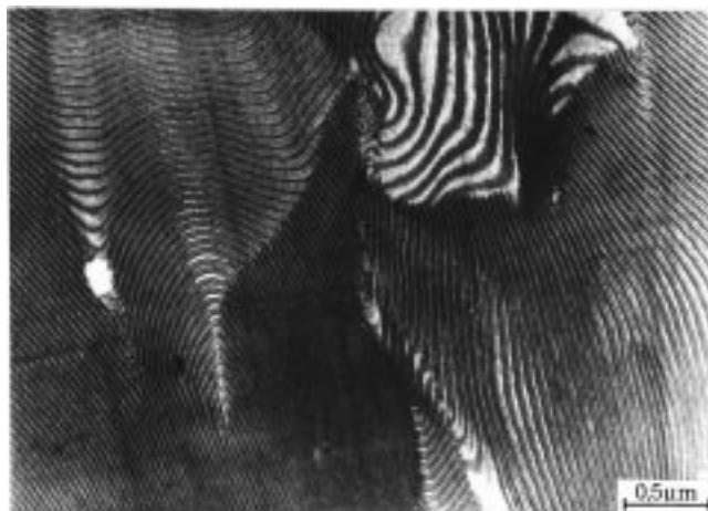
Figure 1. TEM picture of a symmetric P(S- b -nBMA) diblock copolymer stained with RuO 4 .
